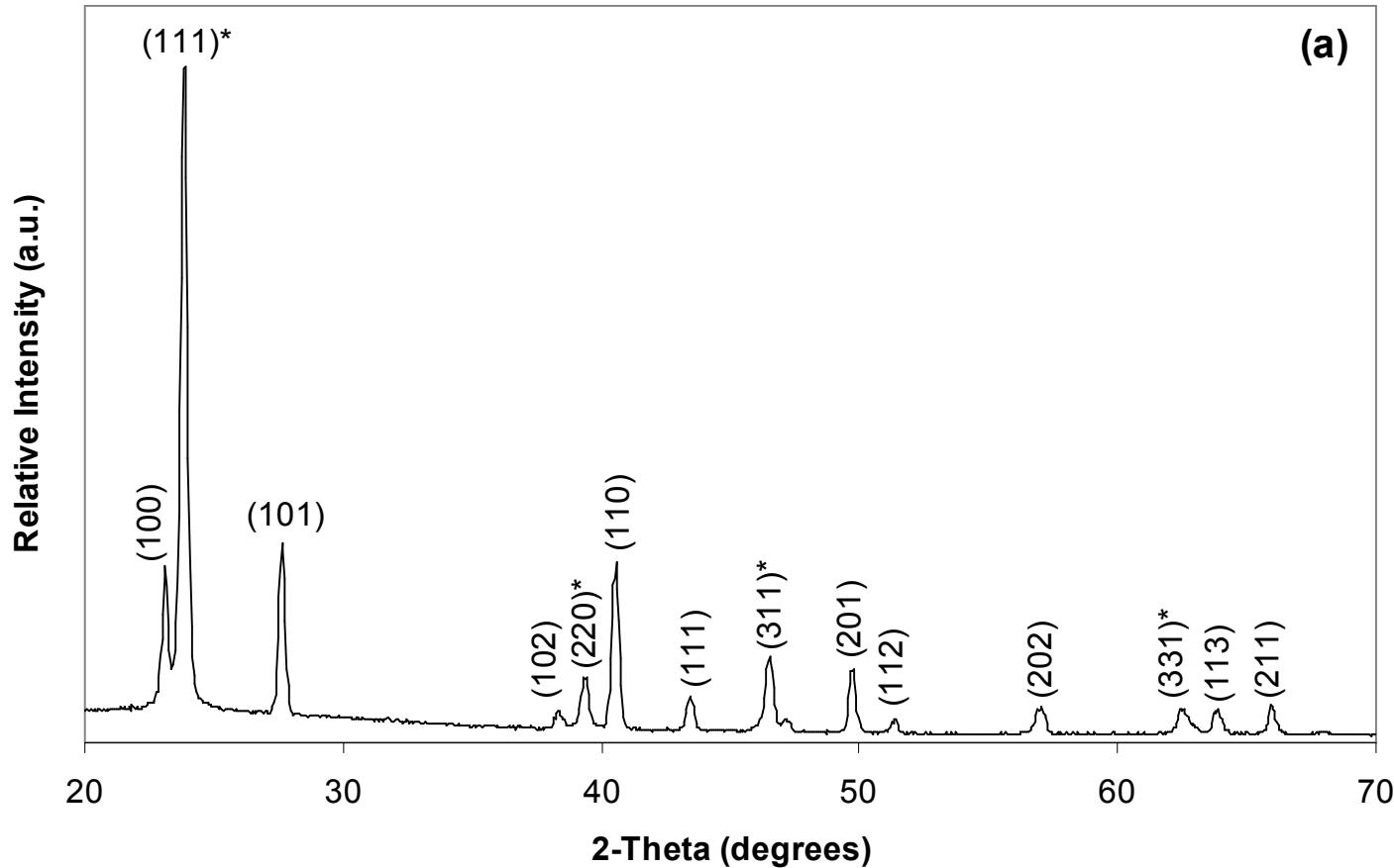
Cubic CdTe marked with asterisk and Hexagonal Te film
