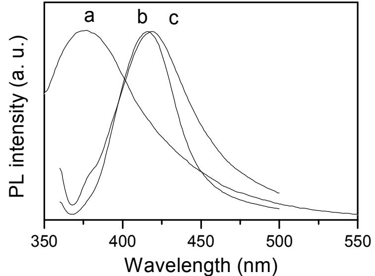
Hexadecylamine (HDA) capped hexagonal ZnSe nanoparticles grown at 300 °C for 30 min from (a) 0.2 g, (b) 0.4 g and (c) 0.6 g of precursor.
