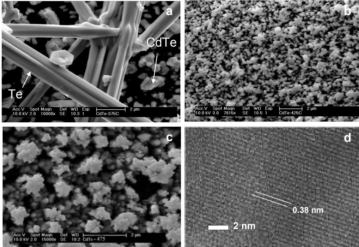
SEM of (a) CdTe and Te deposited at 375°C;
