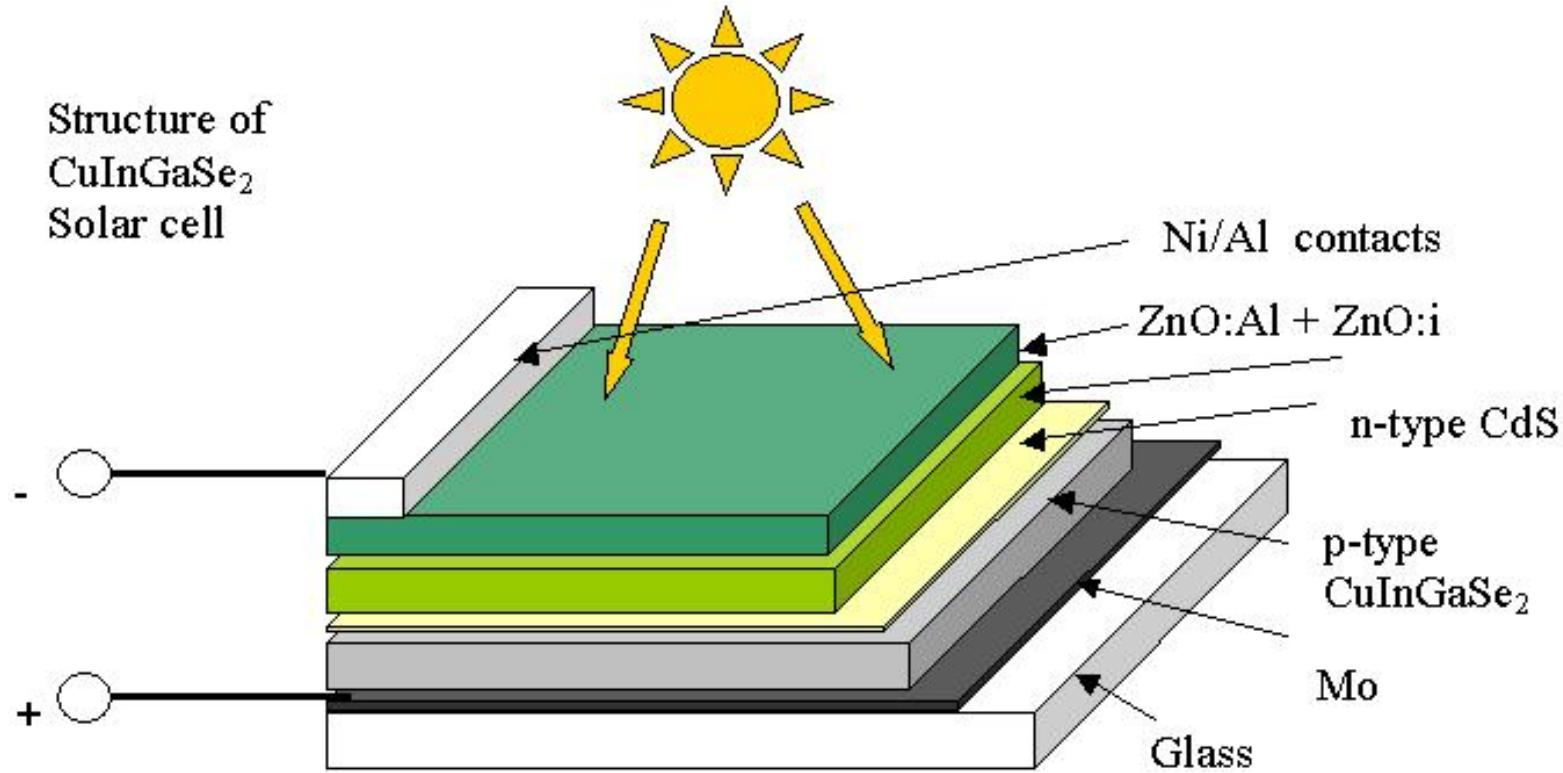
Thin-film solar cells based on CIGS ( $\text{Cu}(\text{In},\text{Ga})\text{Se}_2$ ) companies working with CIGS cells include Shell Solar and Würth.
